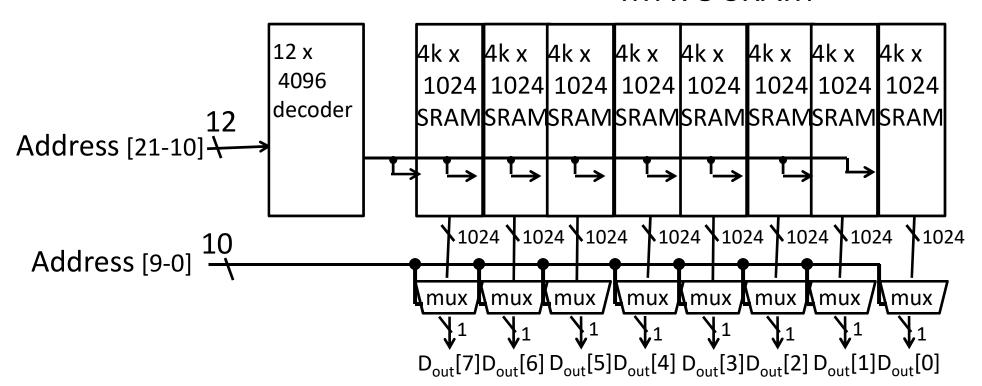
E.g. How do we design a **4M** x **8** SRAM Module?
