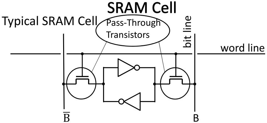
Each cell stores one bit, and requires 4 – 8 transistors (6 is typical)
