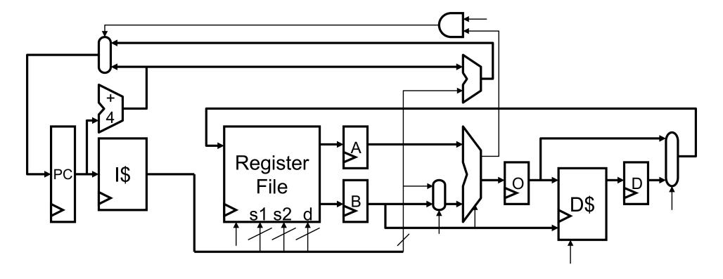
**Multi-cycle datapath**: attacks slow clock Fetch, decode, execute one insn over multiple cycles
