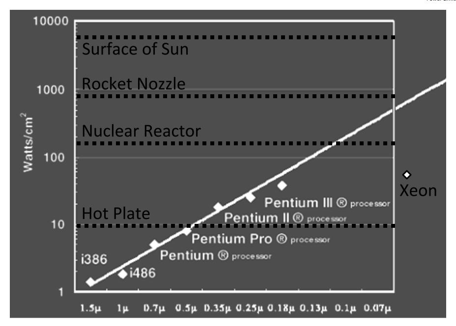
Power = capacitance \* voltage<sup>2</sup> \* frequency In practice: Power ~ voltage<sup>3</sup>
