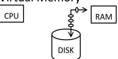
Solution: Pin the page before initiating DMA Alternate solution: Bounce Buffer
