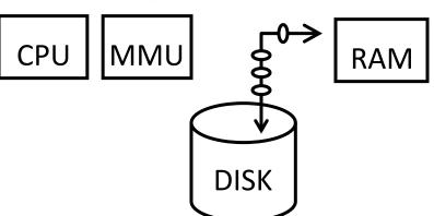
Solution: DMA uses physical addresses
