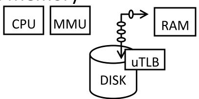
Solution 2: DMA uses virtual addresses
