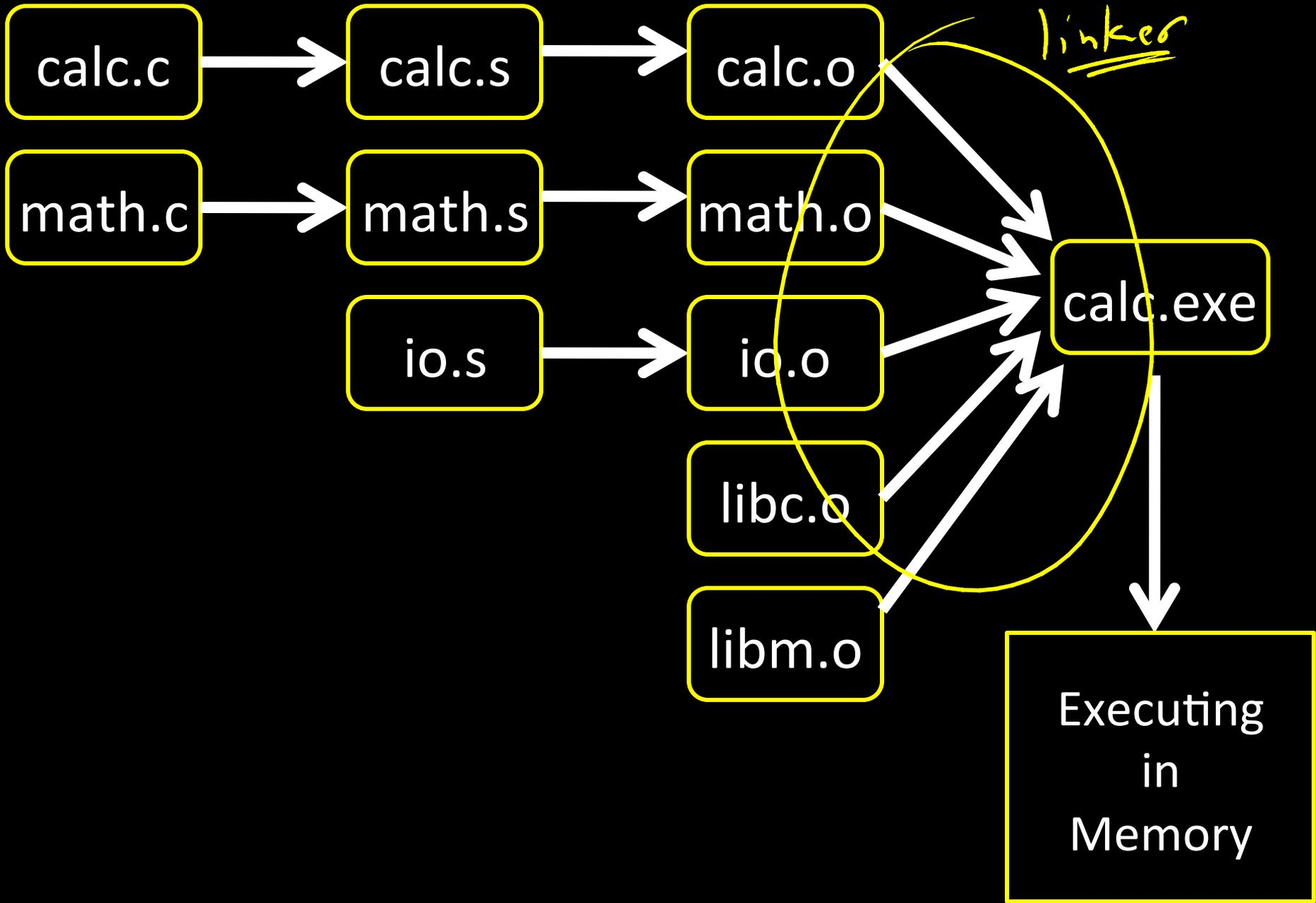
**Linker** combines object files into an executable file
