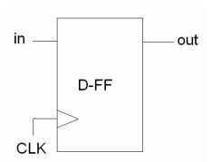
On a positive edge of the clock signal, the D Flip-flop passes the input value to the output.
