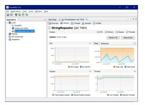
The monitor tab provides a quick, high-level overview of the state of your program. Here, you can see CPU and memory usage in real time.
