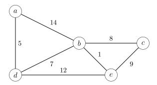
Execute Dijkstra's shortest-path algorithm on the graph above with a as the start node. We show the initial state, before iteration 0 of the main loop, in the second column below, giving the frontier set (the blue set in the description of Dijkstra's algorithm given in lecture), and the L value for each node so far.
