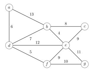
List the edges of the graph above in the order they would be added to a minimum spanning tree by Kruskal's algorithm. If a starting node is required, start with node a. An edge should be listed by the pair of vertices it joins. For example, the edge with weight 12 above would be edge (d, e)
