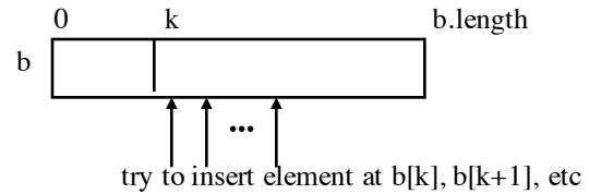
Each test of an array element to see whether it is null or the String is called a **probe**.
