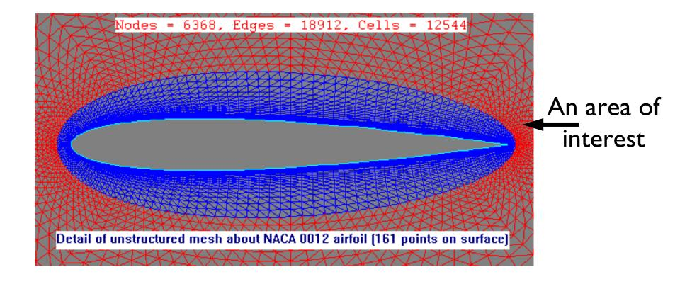
Step one in simulating flow around an airfoil is to generate a mesh and (say) estimate velocity at each mesh point.
