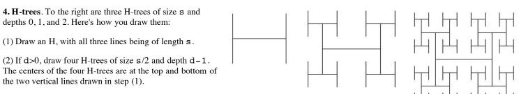
H-trees are useful in designing microprocessor chips. The lines are wires that connect circuit components in a tree of interconnections, without wires crossing.
