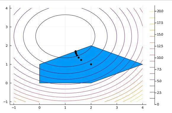
The parameter  $\gamma$  is adjusted dynamically during the solve, and is usually written as  $\gamma = \sigma \mu$  where  $\sigma \in [0,1]$  is the centering parameters and  $\mu = y^T \lambda/m$  is the complimentarity measure, which should go to zero as we approach a problem solution. Getting all the details right is somewhat complicated, though, and we recommend using a package written by someone with some expertise.
