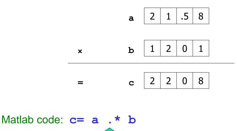
Vectorized element-by-element arithmetic operations on arrays
