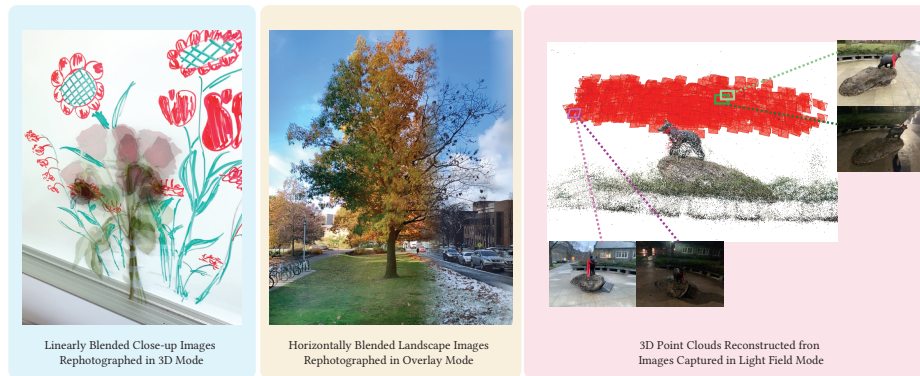
Figure 15: Sample Visualizations of Data Acquired With Each of ReCapture's Three Capture Modes: (left) Wilting roses captured in 3D Mode, which supports accurate multi-view recapture for close-up objects. (middle) A time-lapse image composite of data taken in Overlay Mode, which facilitates robust recapture of more distant scenes (e.g., landscapes). (right) Images showing the estimated poses of a subject captured with Light Field Mode, which helps users capture data for synthesizing new views and 3D reconstruction. See additional results on our project website .
