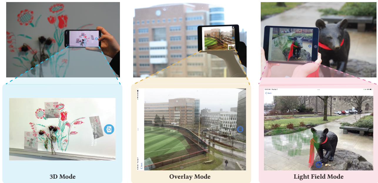
Figure 4: Three Recapture Modes in ReCapture : On the left is 3D Mode, designed for recapturing close-up scenes in situations where tracking and re-registration both work. In the middle is Overlay Mode, which offers guidance in the form of a simple target image overlay for capturing landscapes or scenes where tracking and re-registration fail. On the right is Light Field Mode, which helps users capture a dense range of views and is effective in situations that call for high precision recapture but re-registration fails, or for capturing dense image data to use in image-based reconstructions of the scene.
