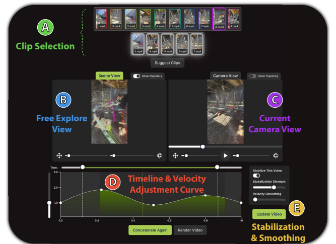
Fig. 4. Editing Interface : Our editing interface has five basic elements: the top Clip Selection (A) part for selecting and ordering candidate clips, the left scene view (B) for a third-person view of the scene and camera trajectories, the right scene view (C) for the current camera view, the timeline window (D) for adjusting camera velocity and trimming the video, and the stabilization and smoothing controls (E) for adjusting camera pose and velocity smoothing. This screenshot shows the interface being used to edit three concatenated clips, but the user can alternatively select individual clips to edit prior to concatenation using the same interface.
