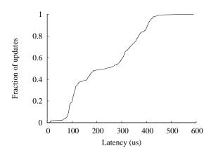
Fig. 6: The cumulative distribution of latencies for updates forwarded by N-BGP operating as a proxy ESM.
