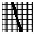
Each row still has a triple of adjacent sub-pixels turned on, so the line still looks white overall, even though the colors that are stored in the pixels are not white.
