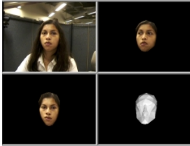
Figure 4-3: Output of the head-tracker based on SFM - clockwise from top left (a) input image (b) tracked head (c) candidate head model (d) frontal warp
