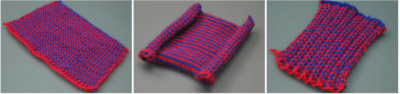
Figure 3: Views of three knitted samples: Note the large differences in dimensions for the same number of stitches and length of yarn. The predictions of our model (Figure 1) are qualitatively similar.
