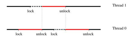
Allow only one process at a time in *critical section* (red). Synchronize using locks, aka mutexes (*mutual exclusion vars*).
