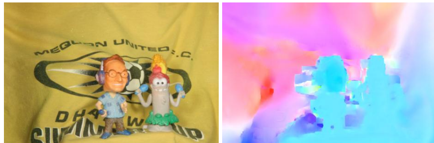
Fig. 4. Output of our model for the sequence “Mequon”. Left: A frame of the image sequence. Right: Estimated flow. Most of the errors occur in the shadows around the cartoon models, due to their high relative motion with respect to the background
