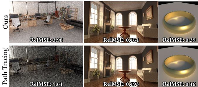
Fig. 10. Equal-time (30s) comparison between the path graph with n indirect samples and m direct samples (top row), and path tracing with m samples (bottom row). The sample count m is determined by the speed of the path tracer, and then n is computed so that the two methods take the same time to run; this provides a comparison with similar quality direct lighting. The path graph is generally more efficient in scenes dominated by indirect lighting, and this comparison shows the transition to where path tracing is more efficient when lighting becomes more direct.
