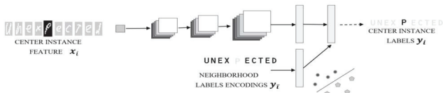
Illustration of ConvPP learning process in 1-D structured labeling tasks (OCR)
