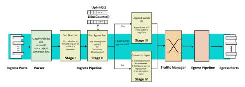
Figure 3: Harmony can be realized using programmable switches supporting PSA architecture. More description on §4.
