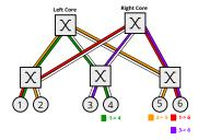
Figure 2: **Understanding benefits of virtual links and host slots. (left)** without multiple virtual links, network may be underutilized due to switches making uncoordinated decisions; and (**center**) without multiple host slots, network may be underutilized due to hosts making uncoordinated decisions; (**right**) using multiple virtual links and host slots, Harmony alleviates network underutilization. Discussion in §3.1.
