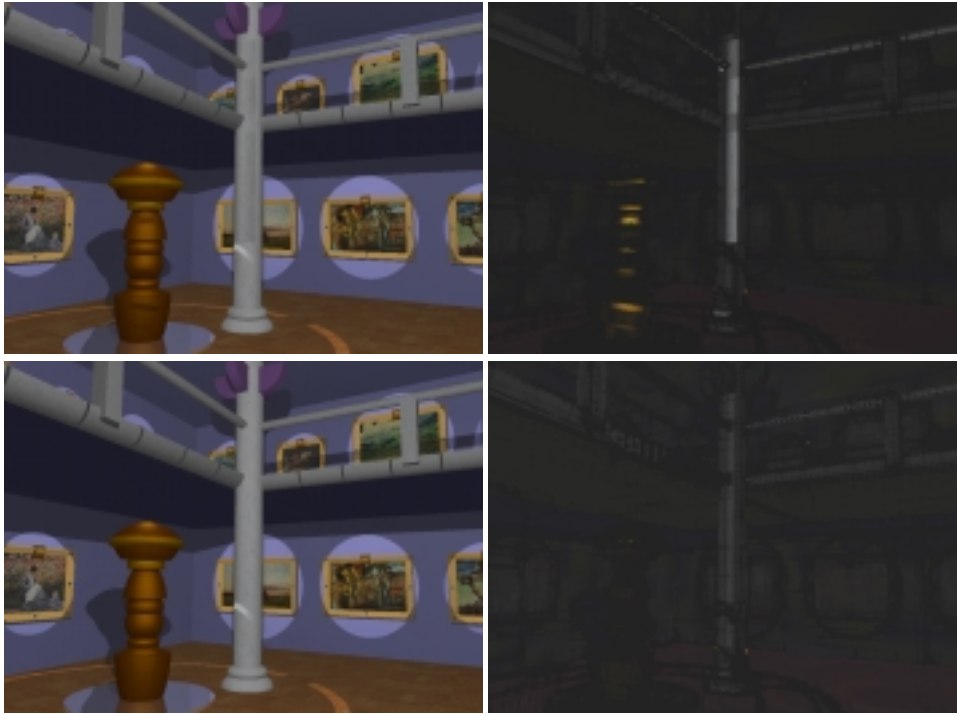
Fig. 15. Error refinement for museum scene. Top row: without non-linearity detection. Bottom row: with non-linearity detection and \epsilon = 0.5 . Right column: scaled difference images.
