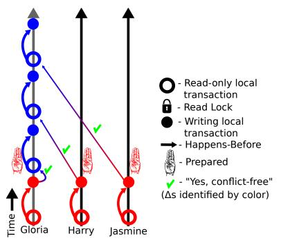
(Here I do not show read locks, but they can be considered to be set just after an SWLT's read and removed just after its write)
