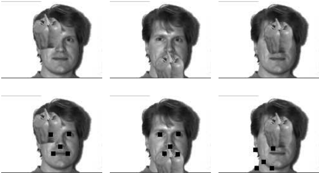
Figure 5: Matching results on occluded faces. The top row shows some input images and the bottom row shows the corresponding matching results. The MAP estimate was a good match when the faces had up to two of five parts occluded and incorrect when three parts were occluded.
