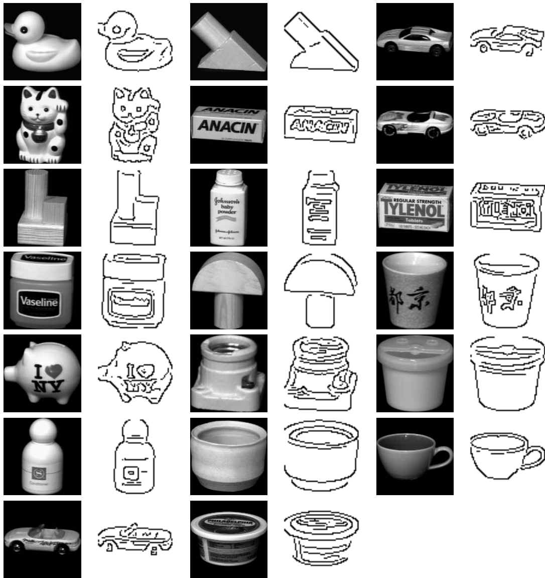
Figure 3: A single view of each of the objects and the edges found in each view.
