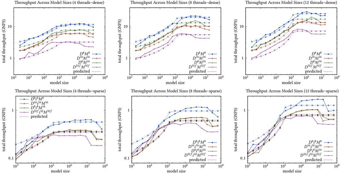
**Figure 3: Comparison of real measured dataset throughput (giga-numbers-per-second) with throughput predicted by the performance model, for multiple threads and precisions, and for sparse and dense data.**
