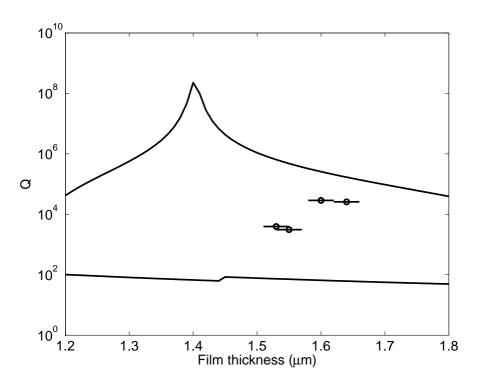
Data from a set of  $30\mu m$  radius disks.
