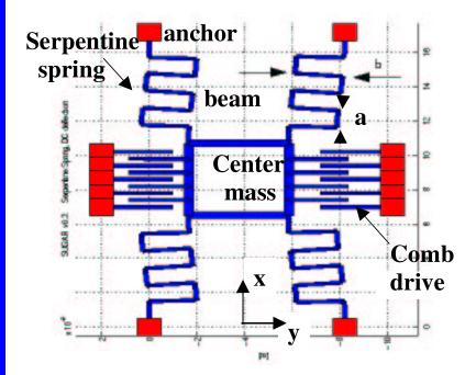
(a) MEMS resonator with four meandering springs
