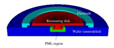
Finite element eigenvalue problem with absorbing layer. Matches experimental results, gives useful predictions.
