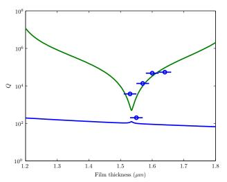
Simulation and lab measurements vs. disk thickness
