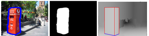
Figure 5: Handling foreground objects: (a) original with segmentation outline, (b) alpha-matte of foreground object, (c) depth map with impostor geometry in the foreground. The red and blue strokes were added for better visibility of the billboards.
