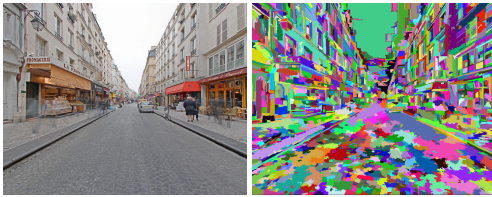
Figure 2: (a) Original image, and (b) superpixels, small segments with uniform color or texture. Our goal is to estimate the 3D location and orientation of the plane on which each superpixel lies.
