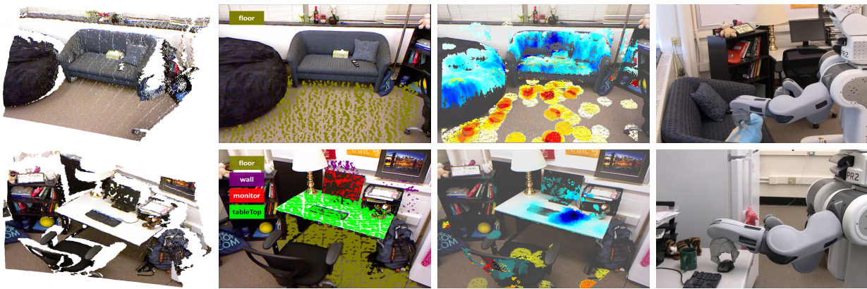
Fig. 17: Robotic experiment (from left to right): (a) A given scene is perceived as a RGB-D point-cloud; (b) The robot uses ILCRF to detect objects; (c) The robot uses ILCRF to infer possible human poses (shown in red heatmaps) and possible placements (shown in blue heatmaps) for placing a cushion (top) and a mouse (bottom) in the scene; (d) The robot successfully places objects in the predicted locations.
