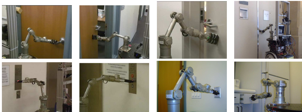
Fig. 6. Snapshots of our robot opening doors and performing several other manipulation tasks.
