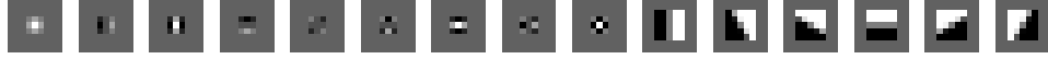
Figure 1: The convolutional filters used for texture energies and gradients. The first nine are 3x3 Laws' masks. The last six are the oriented edge detectors spaced at 30^\circ intervals. The nine Law's masks are used to perform local averaging, edge detection and spot detection.
