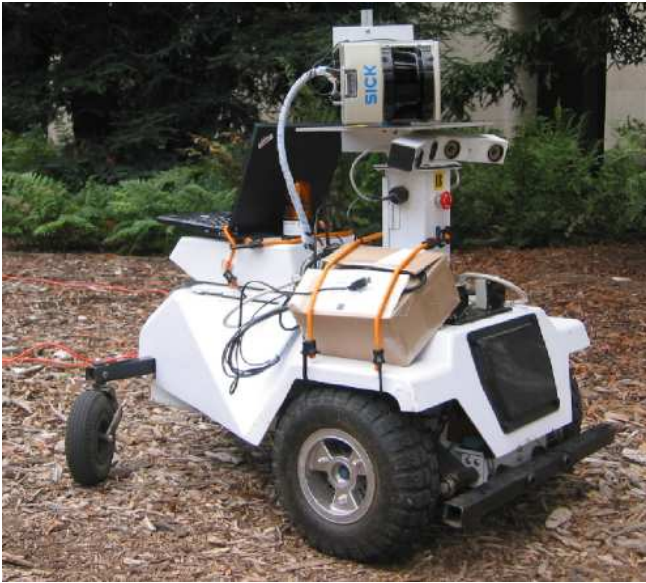
Figure 6: The custom 3-d scanner to collect stereo image pairs and the corresponding depthmaps.
