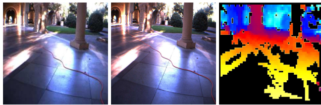
Figure 1: Two images taken from a stereo pair of cameras, and the depthmap calculated by a stereo system. Colors in the depthmap indicate estimated distances from the camera.
