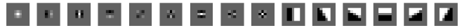
Figure 2: The filters used for computing texture variations and gradients. The first 9 are Laws’ masks, and the last 6 are oriented edge filters.
