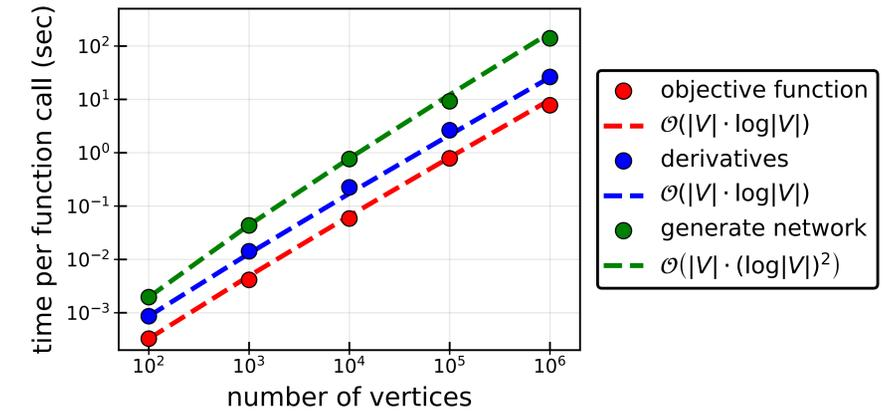
Scalability testing of our fast algorithms on a family of synthetic networks. The **observed timings** are scattered with **circles**, which agrees very well with the **ideal efficiencies** plotted in **dashed lines**.
