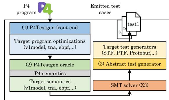
Figure 1: The P4Testgen test case generation process.
