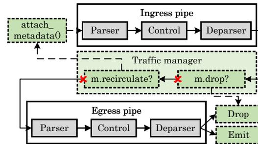
(b) P4Testgen control-flow. Dashed segments are target-defined. `X` is false
