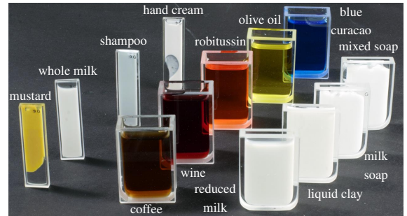
Figure 7: Measured materials in glass cells of width w = 1, 10 , and 2.5 mm, from left to right. It is not necessary for all of the cell to be filled, as long as there exists a homogeneous region of size comparable to the beam diameter (e.g., hand cream).
