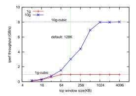
Figure 6: TCP Window Size and Throughput
