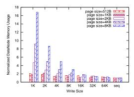
Figure 12: DataNode Memory Overhead
