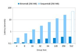
Figure 2.8: Total time for replicating a 256MB object to a large number of nodes on Sierra. than for its actual performance.
