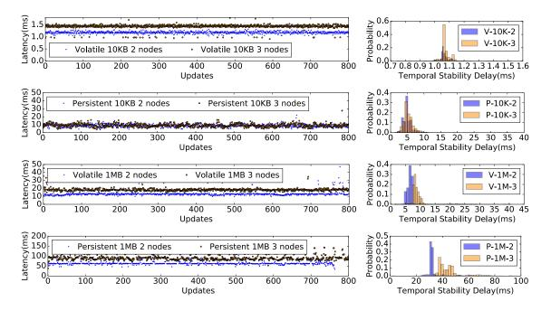
Figure 3.17: End to end performance. On the left, time from when an update was initiated until the new version is temporally stable. On the right, minimum delay for a query to access data at time "now".
