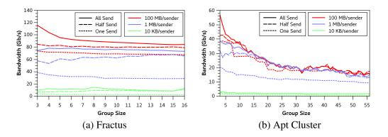
Figure 2.10: Aggregate bandwidth of concurrent multicasts on Fractus and the Apt cluster for cases in which we varied the percentage of active senders in each node-group (in a group with k senders, we used k overlapped RDMC groups with identical membership). The Apt cluster has an oversubscribed TOR; our protocols gracefully adapt to match the available bandwidth.
