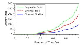
Figure 2.9: Distribution of latencies when simulating the Cosmos storage system replication layer.
