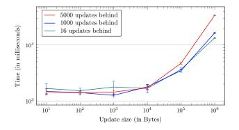
Figure 5.6: Time to restart a service with 3 shards of 3 members each, with 1 out-of-date node per shard. Error bars represent 1 standard deviation.
