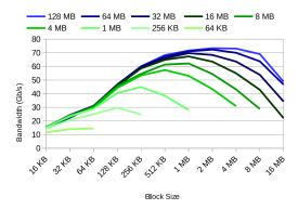
Figure 2.6: Multicast bandwidth (computed as the message size divided by the latency) on Fractus across a range of block sizes for messages between 16 KB and 128 MB, all for groups of size 4.
