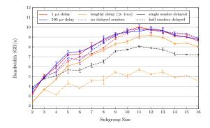
Figure 4.10: Data for sender delay test with null-sends.
