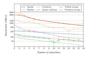
Figure 4.18: DDS performance improvements with Spindle optimizations for all 4 QoS levels.
