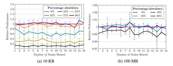
Figure 3.19: Derecho performance for various values for efficiency and number of slow nodes, as a fraction of the no-slowdown case.
