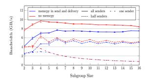
Figure 4.15: Performance with memcpy in send and delivery.
