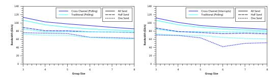
Figure 2.12: CORE-Direct experiment using a chain multicast protocol to send a 100 MB message. The left is a run using hybrid polling/interrupts; on the right is a run with purely interrupts. Both experiments were on Fractus.
