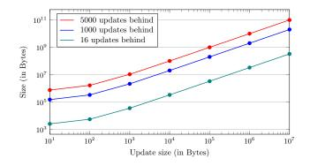
Figure 5.5: Data downloaded by each out-of-date node, in a system with 3 shards of 3 members each.
