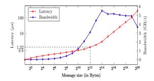
Figure 4.14: Performance of memcpy with data size.
