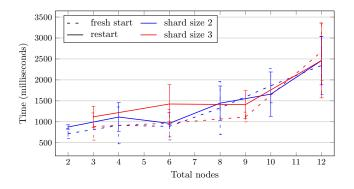
Figure 5.2: Total time to start or restart a service. Error bars represent 1 standard deviation.
