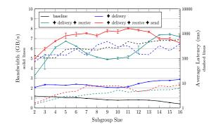
Figure 4.5: Performance gains with batching applied to successively more stages of the pipeline for all senders. Throughput (left Y-axis) is shown by solid lines, and latency (right Y-axis) using dashed lines. Both metrics show significant improvements relative to our baseline system.
