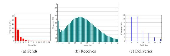
Figure 4.7: Batching histograms for the three protocol stages. Receive merges data streams from all senders, forming larger batches. Delivery computes an extra level of stability over all members, forming even larger batches.
