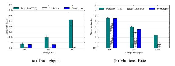
Figure 3.23: Derecho vs LibPaxos and ZooKeeper with Three Nodes over 100Gbps Ethernet
