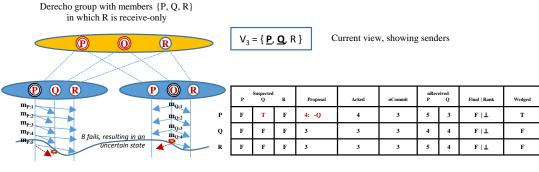
RDMC groups for senders P and Q. If Q fails, the group wedges along the ragged blue line, disrupting  $m_{P:5}$  and  $m_{Q:4}$ .
