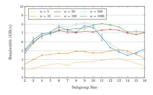
Figure 4.6: Performance with different window sizes when all nodes are sending messages continuously
