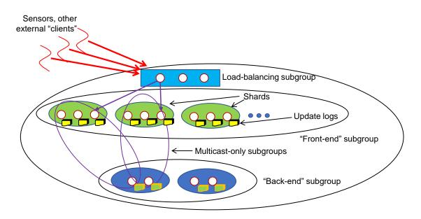
Figure 5.1: A Derecho service spanning 16 (or more) machines and containing several subsystems that employ a mix of point-to-point RPC and multicast. The ovals represent subgroups and shards within which data is replicated. Independent use of state machine replication isn't sufficient: after a shutdown, components must restart in a *mutually-consistent* state.
