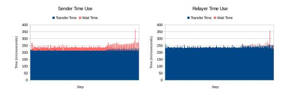
Figure 2.5: Breakdown of transfer time and wait time of two nodes taking part in the 256 MB transfer. The majority of time is spent in hardware (blue), but the sender (left) incurs a higher CPU burden (orange) than the receiver (right). Offloading RDMC fully into the hardware would eliminate this residual load and reduce the risk that a long user-level scheduling delay could impact overall transfer performance.
