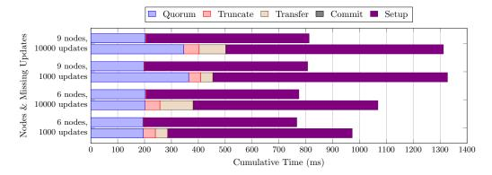
Figure 5.4: Breakdown of time spent in each phase of starting or restarting a service, when 1 node per shard is out of date upon restart. Upper bars show fresh start, lower bars show restart.
