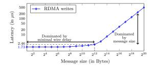
Figure 4.1: Latency vs data size on 100 Gbps Mellanox RDMA. Latency is nearly constant for up to 4KB message size.
