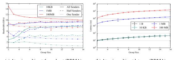
(a) Atomic multicast throughput (RDMA)(b) Atomic multicast latency (RDMA)Figure 3.12: Derecho's RDMA performance with 100Gbps InfiniBand
