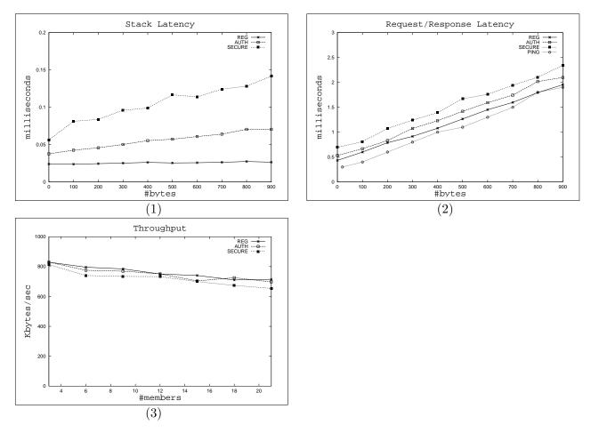
Figure 1: A standard stack is denoted REG. An authenticated stack is denoted AUTH. An authenticated encrypted stack is denoted SECURE. (1) send-recv latency in the Ensemble stack. (2) Total Latency for point-to-point send/recv. (3) Throughput.
