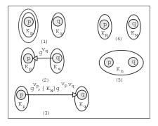
Figure 3: A variation on the merge sequence that guarantees PFS. (1) Two components with keys  $K_p$  and  $K_q$ . Each leader sends IamAlive messages. (2) q sends  $g^{v_q}$  to p. (3) p chooses a new key  $K_N$ , sends  $g^{v_p}$  and  $K_N$  encrypted with  $g^{v_p v_q}$  to q. (4) q decrypts  $K_N$  and switches his component key to  $K_N$ . Component P switches its key to  $K_N$ . (5) Components P and Q now merge, after both have the same key  $(K_N)$ .
