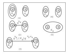
Figure 2: Overview of the merge sequence. (1) Two components with keys  $K_p$  and  $K_q$ . Each leader sends IamAlive messages. (2) q sends  $g^{v_q}$  to p. (3) p sends  $g^{v_p}$  and  $K_P$  encrypted with  $g^{v_p v_q}$  to q. (4) q decrypts  $K_p$  and switches his component key to  $K_p$ . (5) Components P and Q now merge, after both have the same key.
