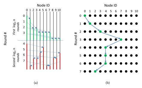
Fig. 1. (a) Information flow from node 0 in our scheme, showing two full epidemic cycles of  $\log_2 n$  rounds each. Every process sends and receives one message per round; we omitted the extra messages to reduce clutter. Similarly, although each round can be viewed as a new epidemic, the figure just shows two. (b) Example of the path taken by a tunneled message from node 0 to node 3. This message would have 5 layers of onion encryption since it has 5 different recipients.
