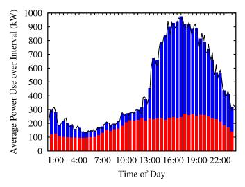
Fig. 5. Data collected by the utility, running queries using our system. Red bars are reported nonshiftable load, while blue bars are reported load from devices with DSM potential (i.e., heating and cooling systems). The black line is the actual consumption recorded by the meters locally.
