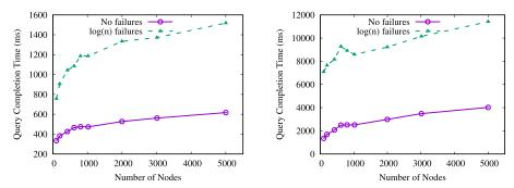
Fig. 6. Time for a single query to complete, in simulated milliseconds for the basic protocol (left) and the BFT variant (right).
