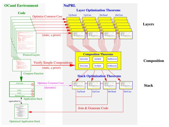
Figure 5. Optimization methodology: composing optimization theorems.
