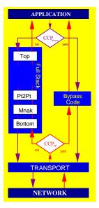
Figure 4. Optimized code architecture from run-time statistics. We call the result of optimizing a
