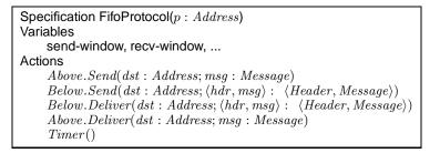
Figure 3. The prototype of a concrete behavioral specification of a communication protocol that retransmits messages, removes duplicates, and delivers messages in order. Each process that participates in the protocol runs an instance of one of these.
