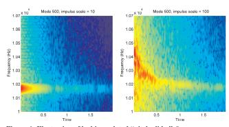
Figure 6: Illustration of locking-related "pitch glide:" Spectrograms are shown for virtual cymbal sounds resulting from different impulse magnitudes. As the impulse magnitude grows, one can see an increasingly noticeable frequency drop at the beginning of the spectrograms.
