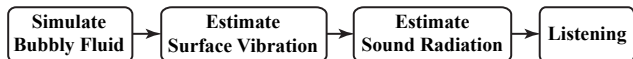
Figure 3: Overview: (1) We first simulate an incompressible fluid flow with bubbles. For each vibrating bubble we (2) estimate the induced fluid-air surface vibration and (3) resulting air-domain sound pressure. (4) Finally, the linear superposition of bubble sound fields are rendered to the listener.
