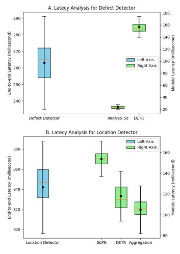
Fig. 3. Sample application latency analysis.
